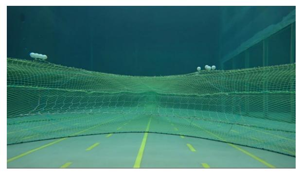
Side view of the killer whale deterrence panel during a simulated haulback and rounder shape of net. Note the panel is well ahead of the footrope and leadlines fill the space below the panel
