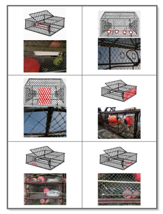
Figure A4-1 Crab pots demonstrating tunnel eye opening, escape rings, escape mesh, and biotwine. Top photos show Tanner boards (left) and escape rings (right). Middle photos show escape mesh. Bottom photos show biotwine examples.
