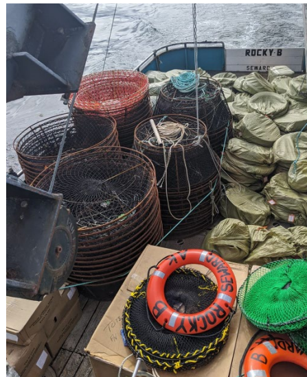
Figure 4-5 Comparison of space required on deck for 60 large, stackable black cod pots (left) and 650 collapsible pots (right). Source: Fish Tech Inc., social media, June 2020.
