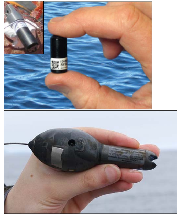
Figure 2.—Size comparison of acoustic tag and satellite tag. Vemco V9 pictured on top with and without end cap (note that tag with end cap is a V9-2, which is 0.5 cm longer than the proposed V9-1). Wildlife Computers MiniPAT pictured on bottom.
