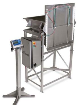
Figure 2-4 Hopper scale. Photo credit: Marel (https://marel.com/en/products/hopper-scales/fish). This image is for example purposes only and does not represent an endorsement by NMFS.
