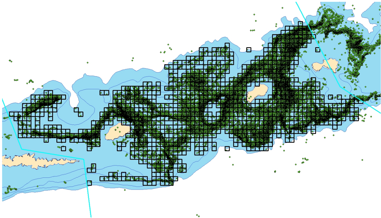
Figure C.1. Survey design: 2 nmi x 2 nmi grids overlaid on observer pot sample locations (green squares) in EAG .
