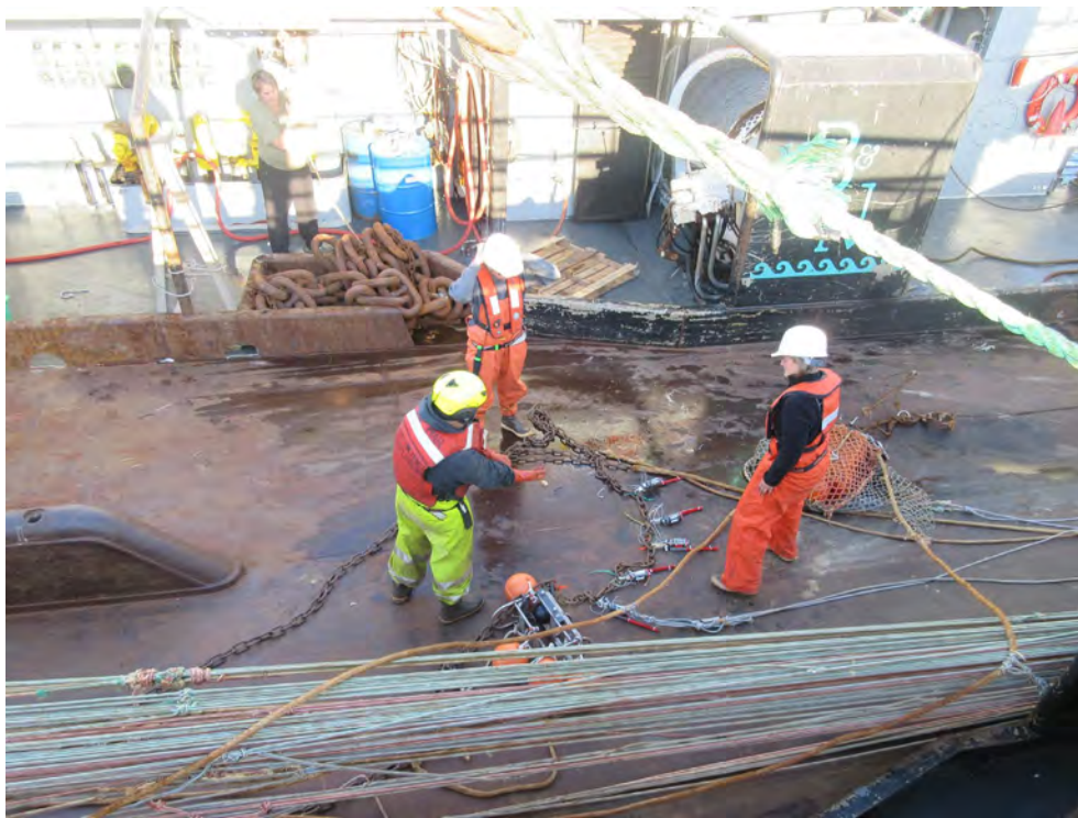
Figure A- 8 Examples of clump weights (top left) and footrope (middle center) used for pelagic trawl gear.
