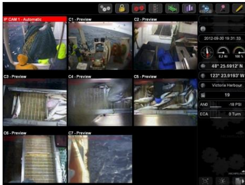
Figure 3 The Archipelago EM system user interface showing camera views, sensor activity and status.
