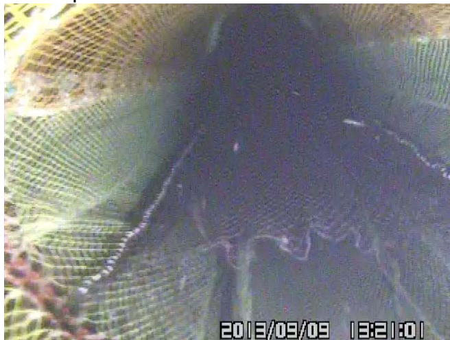
Figure 3. Flapper hanging about half-way down, Alaska Beauty fall 2013. View is looking forward from aft end of excluder in the last tapered section of the Swan net. The elevated hood is seen at the forward end of the excluder’s panel.
