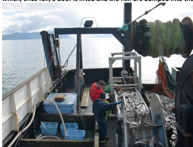
Figure 2. Deck of F/V Caravelle with fish flowing from the trawl alley, across the conveyor belt and into the "weigh" box from which, once full, a door is lifted and the fish are dumped into the hold below. The sea sampler is in the red jacket.
