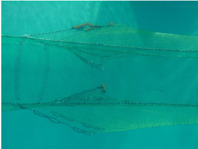
Figure 13. V.2 Over/Under Excluder designs for the Caravelle and Alaska Beauty used during the spring and Fall 2014 EFP trials. The excluder was placed at the aft end of the last tapered section in the Caravelle net, at the forward end of the last tapered section in the AK Beauty net (zero overlap). Cross section is below, showing the larger “scoops” in this design with the goal of increasing the area available for escapement. Video cameras were used to monitor and quantify salmon and pollock escapes.
