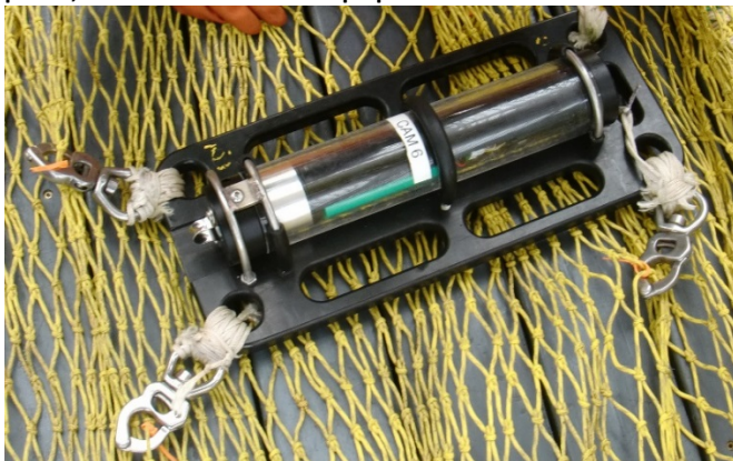
Figure 11. Acrylic tube underwater video camera placed in the net to monitor fish escapes. One was placed near the top portal, one at the bottom escape portal
