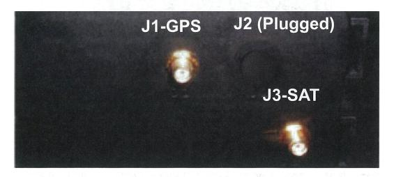
7) Connect the GPS antenna cable to connector GPS (J1) with cable labeled GPS on each end.
