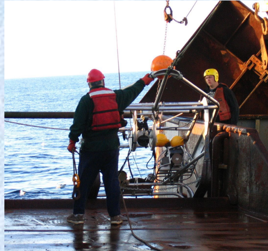
Video and sonar on a sled
