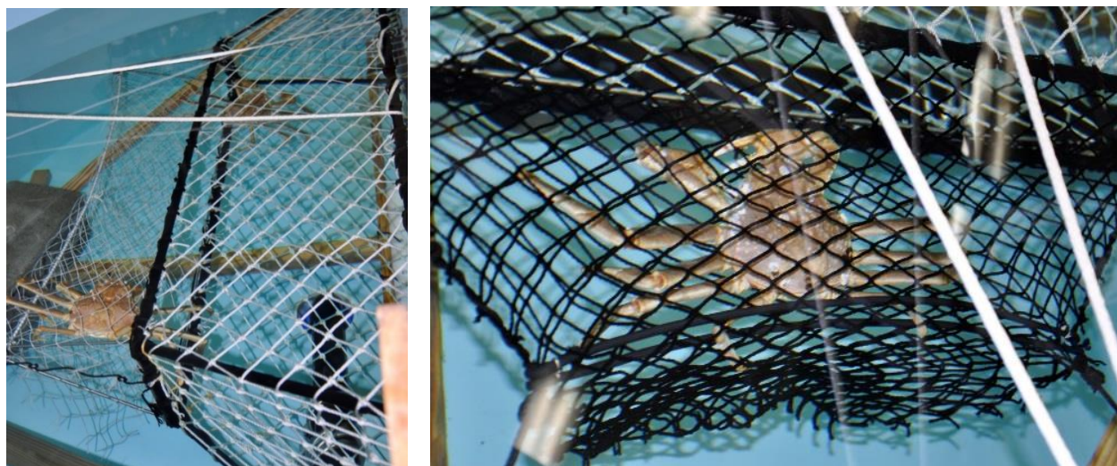
Figure 3. Photos from Kodiak lab trials showing additional opilio test panel variants with the Dyneema sock (right) and 'black sock' (left) tunnel inserts, each with opilio crab approaching passage. Dyneema is a newer, high strength, synthetic fiber material used in some fishing gears.
