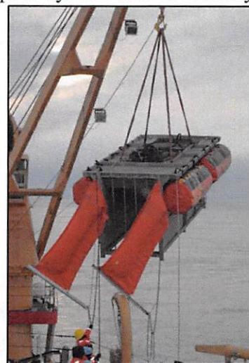
DIP-600 Skimmer Being Deployed
