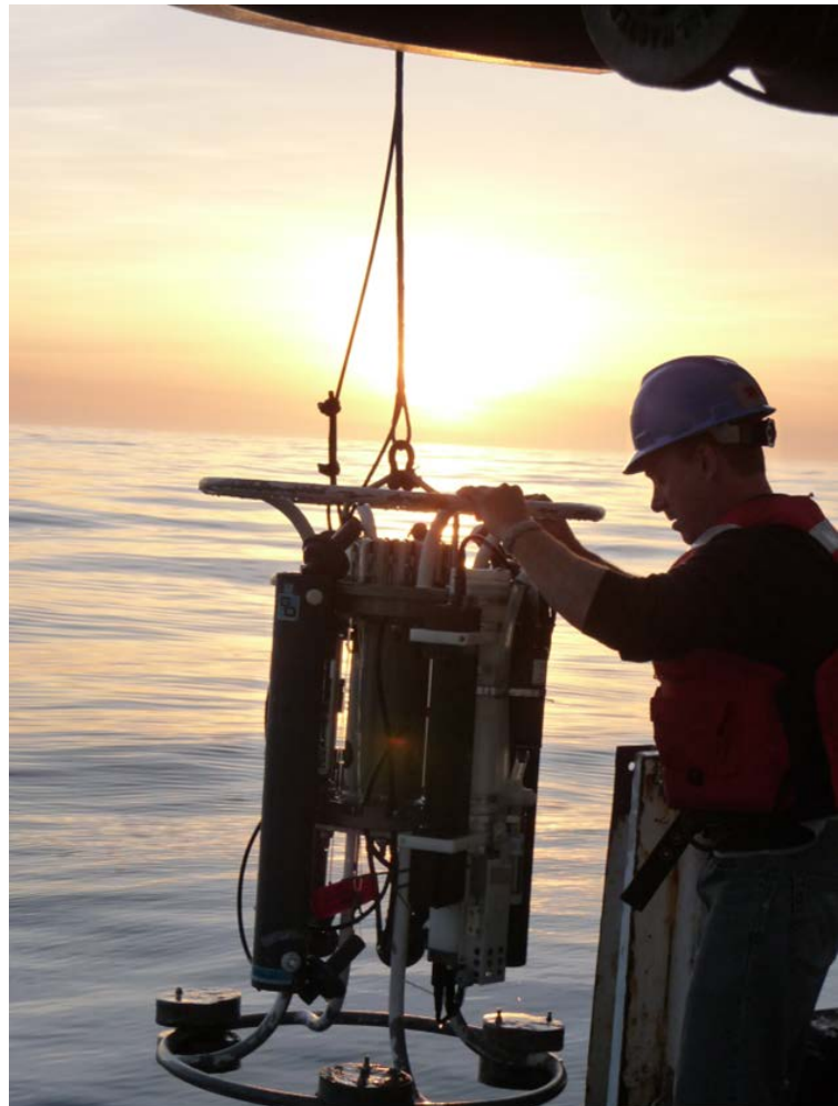
Brian Wells, NOAA SWFSC, lowering CTD (Conductivity-Temperature-Depth) Sensor into Pacific Ocean. Photo credit: NOAA/SWFSC
