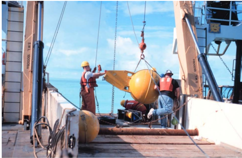
Oceanographic data buoy being deployed from R/V Miller Freeman. Photo credit: NOAA.
