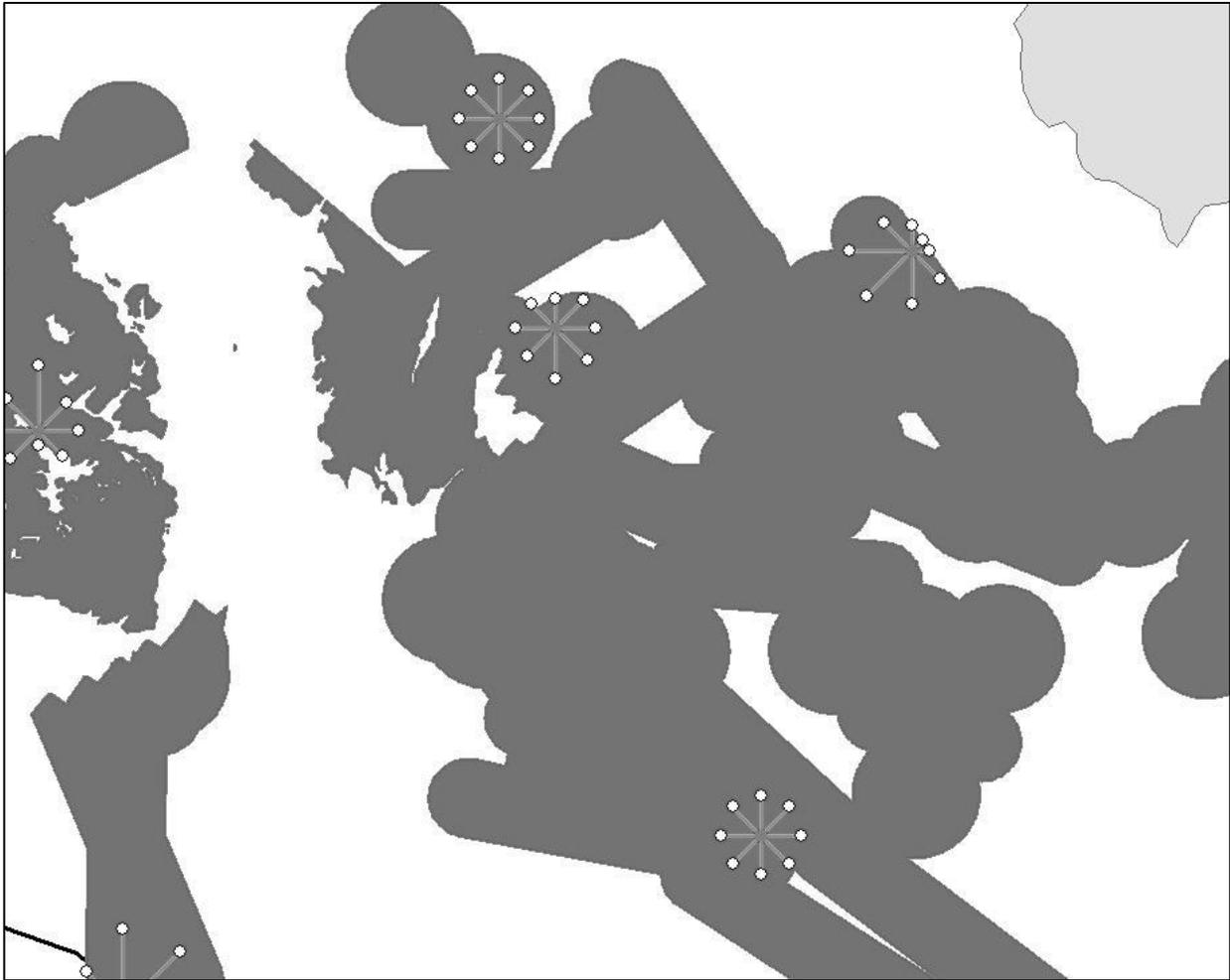
Figure 14.7.—Example of 1-km transect plan lines for remote operated vehicle (ROV) dives. Plan lines have been adjusted in some cases to remain within the delineation of rocky habitat (solid gray).
