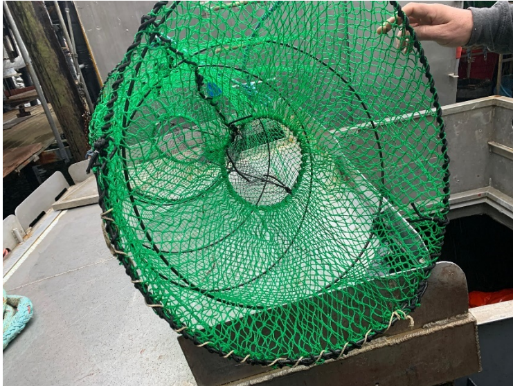
Figure 4-12 Slinky pot with door wrapped closed with cotton twine (white thread on bottom of photo). Proposed in Element 1, currently not allowed by regulation. Source: NMFS OLE, B. Cheeseman.
