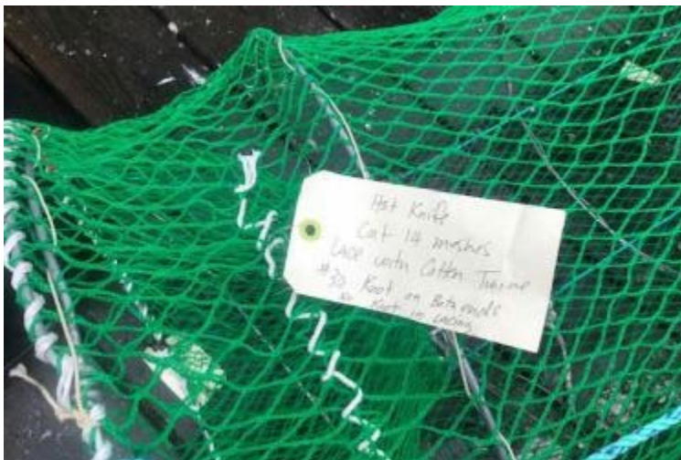
Figure 4-13 Slinky pot with biodegradable twine/panel tied into the mesh of the pot, allowed by status quo regulation. Source: https://www.fisheries.noaa.gov/alaska/commercial-fishing/longline-pot-gear-gulf-alaska-ifq-sablefish-fishery-frequently-asked
