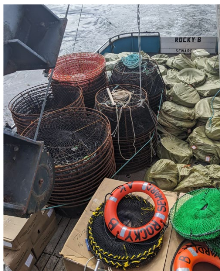
Figure 4-7 Space required on deck for 60 large, stackable black cod pots (left) and 650 collapsible pots (right). Source: Fish Tech Inc., social media, June 2020.
