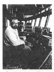
Captain Jack Jones filters information from VHF radios, an echo sounder, two sonars, chart plotters, and a radar screen.
