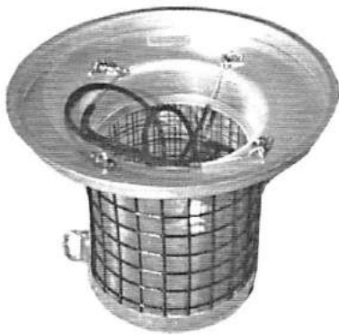
25" Gullywashette - 30 mesh stainless steel wire cloth between 2x2 and 1x1 wire sides. Removable aluminum support frame, fixed aluminum bottom pan, brass handle. Part # 12001
