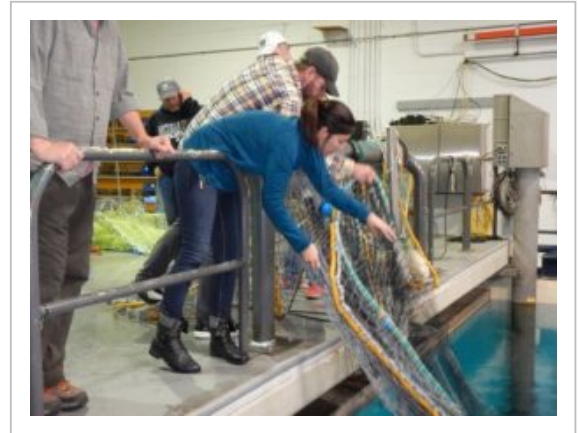
Dropping trawl net with excluder device into flume tank, courtesy John Gauvin
