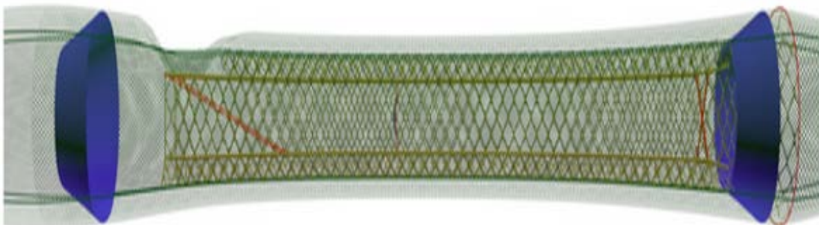
Figure 3: Conceptual depiction of a “hallway” halibut excluder (top view)
