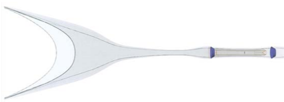
Figure 4: Conceptual drawing illustrating a hallway halibut excluder installed in a flatfish net
