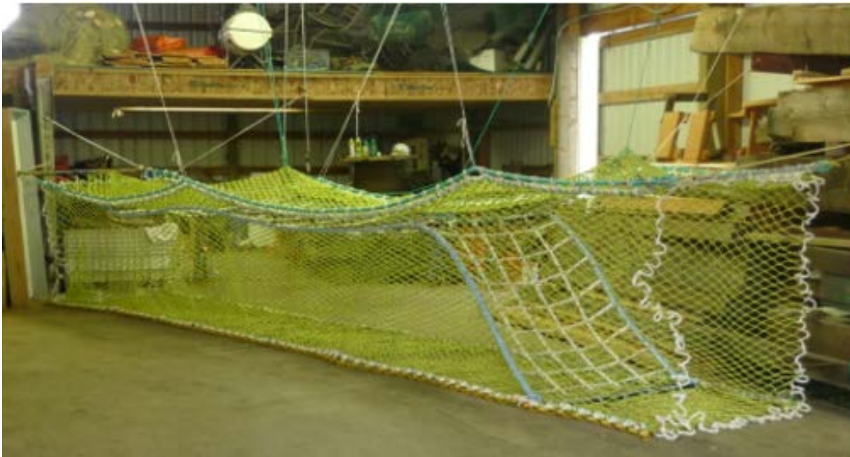
Figure 2: Picture of a semi-rigid (“Pex” grate) salmon excluder
