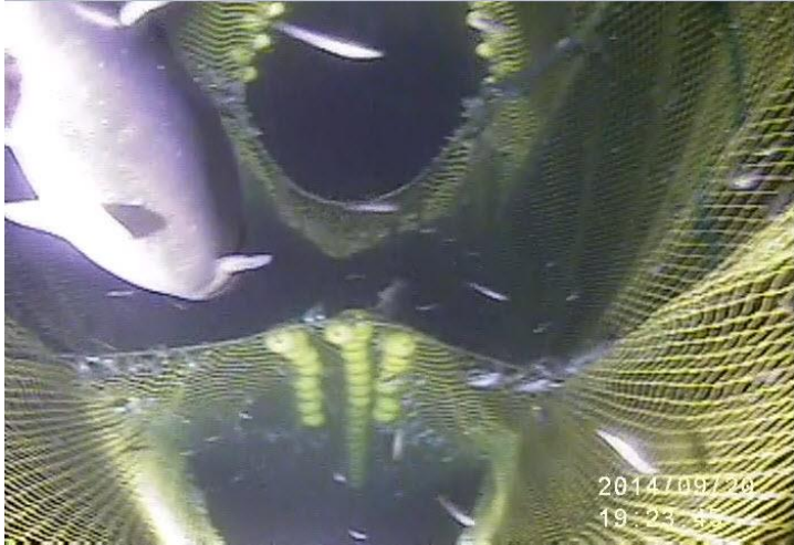
Figure 8. Caravelle O/U excluder, Fall 2014. View is from aft of the excluder looking forward towards the mouth of the net. The large over and under escape portals are clearly shown with a salmon swimming forward towards the bottom escape hole.
