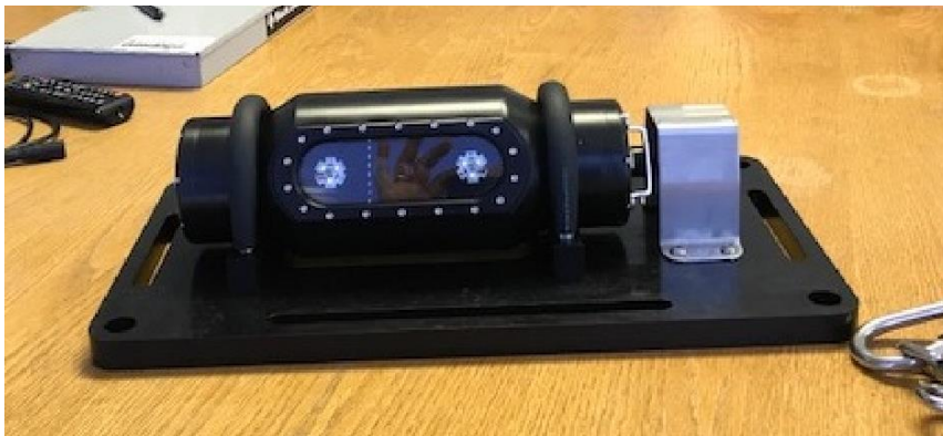
Fig 3 Beta version of the tube camera developed by Williamson and Associates that will be used to quantify salmon and pollock escapement in the proposed EFP research.
