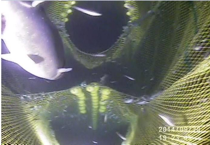
Figure 6. O/U Salmon excluder at depth on the Caravelle, GOA EFP 13-01. The camera is looking forward towards the mouth of the net and a salmon is seen swimming forward to escape out of one of the escape portals.
