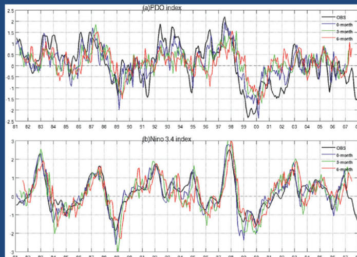
FIG. 5. Time series of (a) the PDO index and (b) the Niño-3.4 SST anomaly during 1981–2006. Black line denotes observation, and blue, green, and red lines denote CFS predictions at 0-, 3-, and 6-month lead, respectively.
