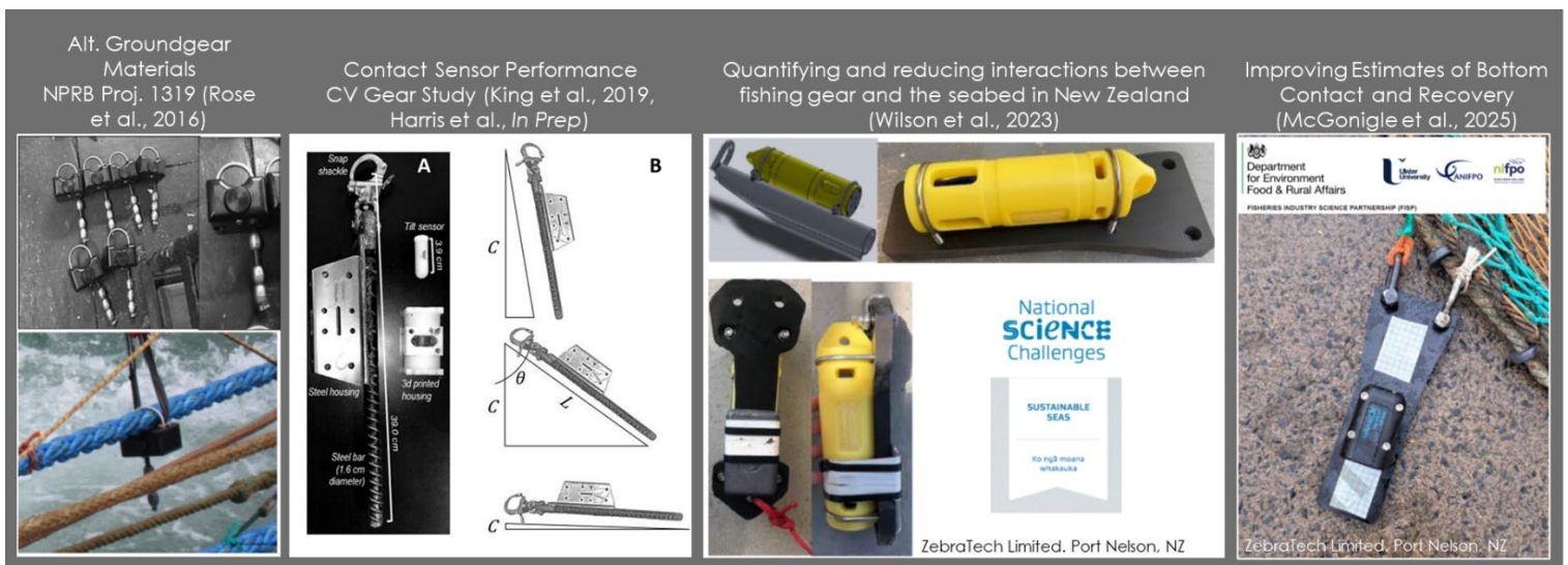
Figure 4. Tilt sensor development to measure bottom contact and seafloor clearance from four projects starting in 2016 through 2025. Every sensor, associated protective housing, and attachment method were different and customized to the research project needs, vessel type, and gear type. (Images source: FAST Lab, 2025).
