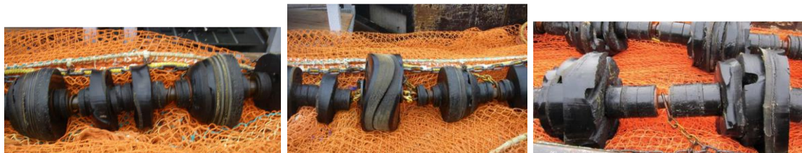
Figure 4 – Four footrope designs used to study unobserved mortality of Bering Sea crabs: Left - 16" bobbin and disk, Middle - 16" footrope raised by inserting 21" disks, Right - 24" disks and bobbins.
