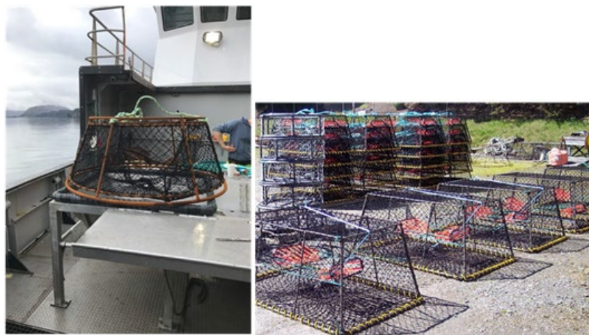
Figure 3-7 Examples of stackable (left) and trapezoidal (right) groundfish pots
