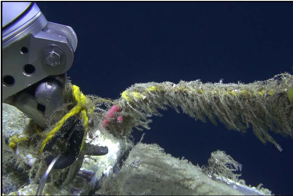
Figure 13. Retrieval of array # 8 at Site 4 (Fairweather Ground) showing heavy growth of hydroids after a 22-month deployment.
