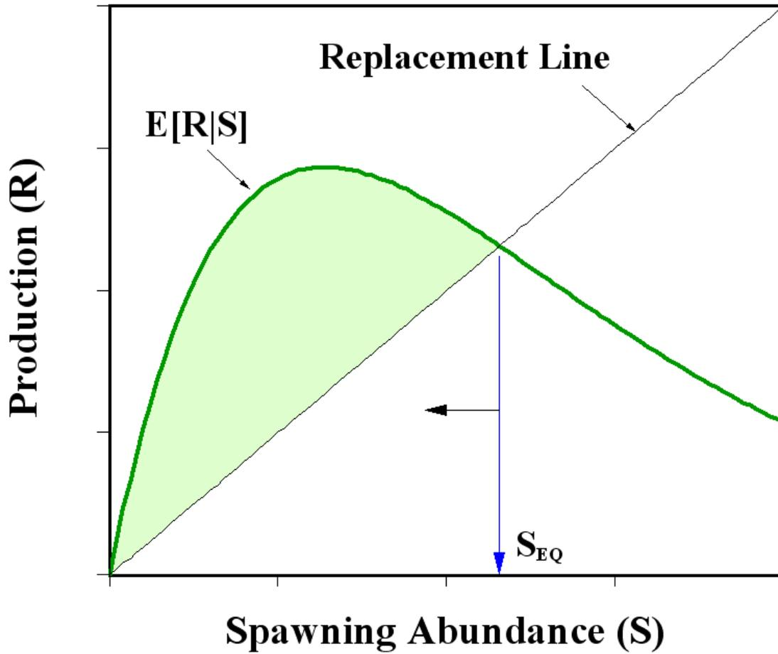
Figure 4. Schematic of the Ricker production model with potential sustained yields in the shaded area between  $E[R|S]$  and the replacement line ( $R = S$ ) and escapements less than carrying capacity ( $S_{EQ}$ ).  $S_{MSY}$  generally occurs between 29 and 43 percent of  $S_{EQ}$  for Pacific salmon.
