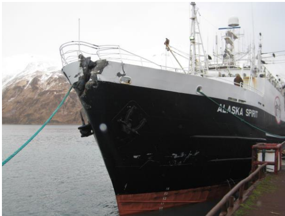
Damage to the Bow of F/V Alaska Spirit
