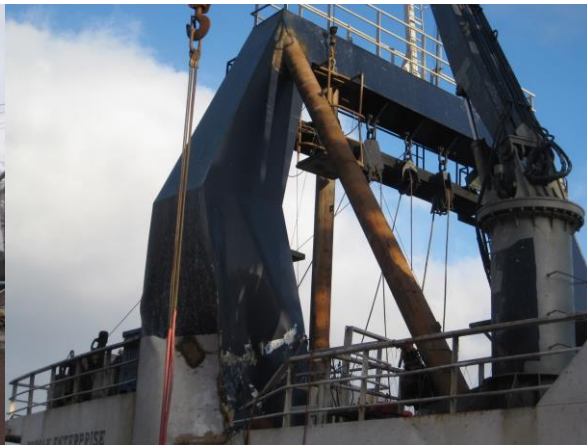
Damage to the gantry of F/V Kodiak Enterprise
